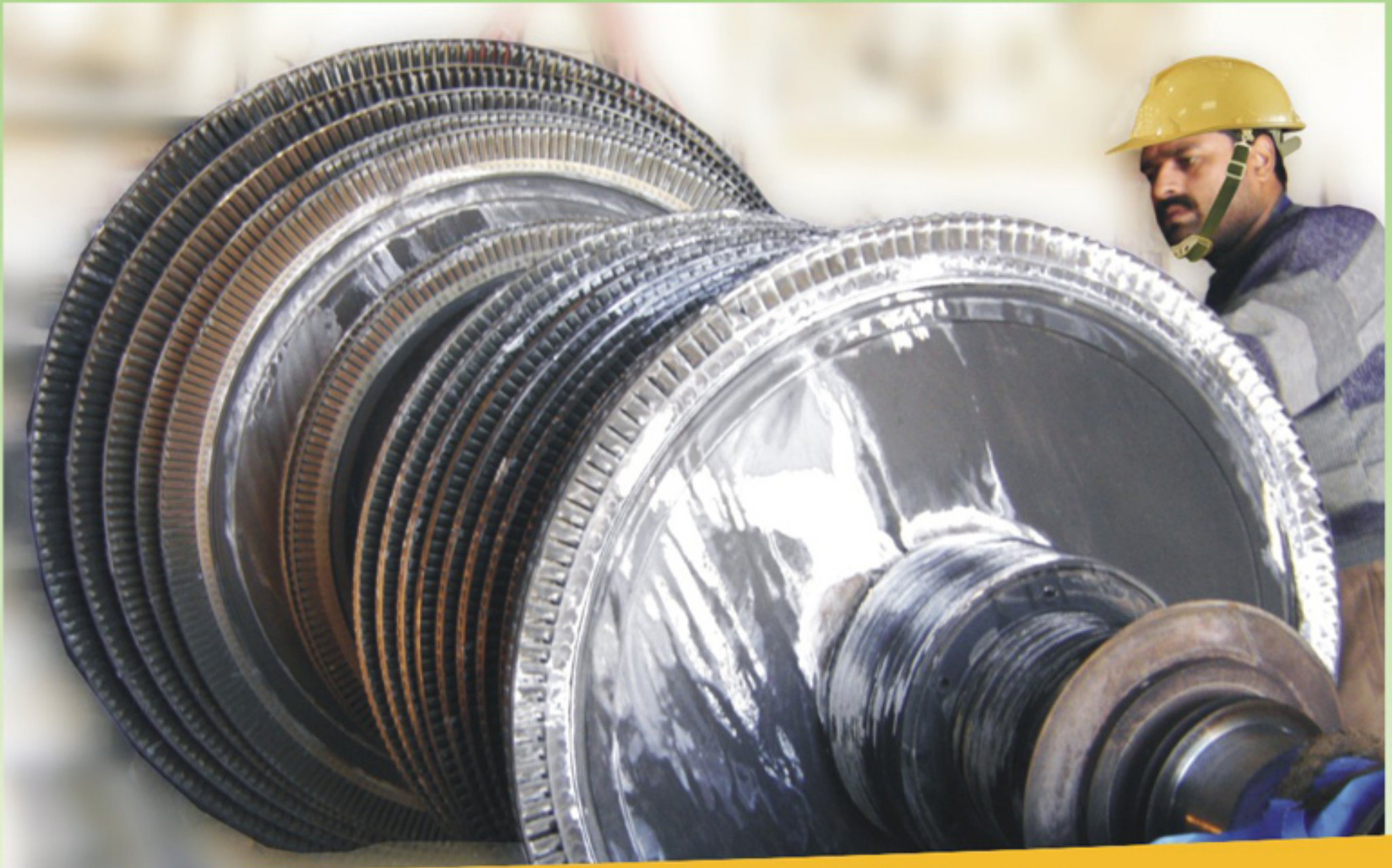
After Repair Multistage Rotor 12000 KW Alnoor Sugar Mills
