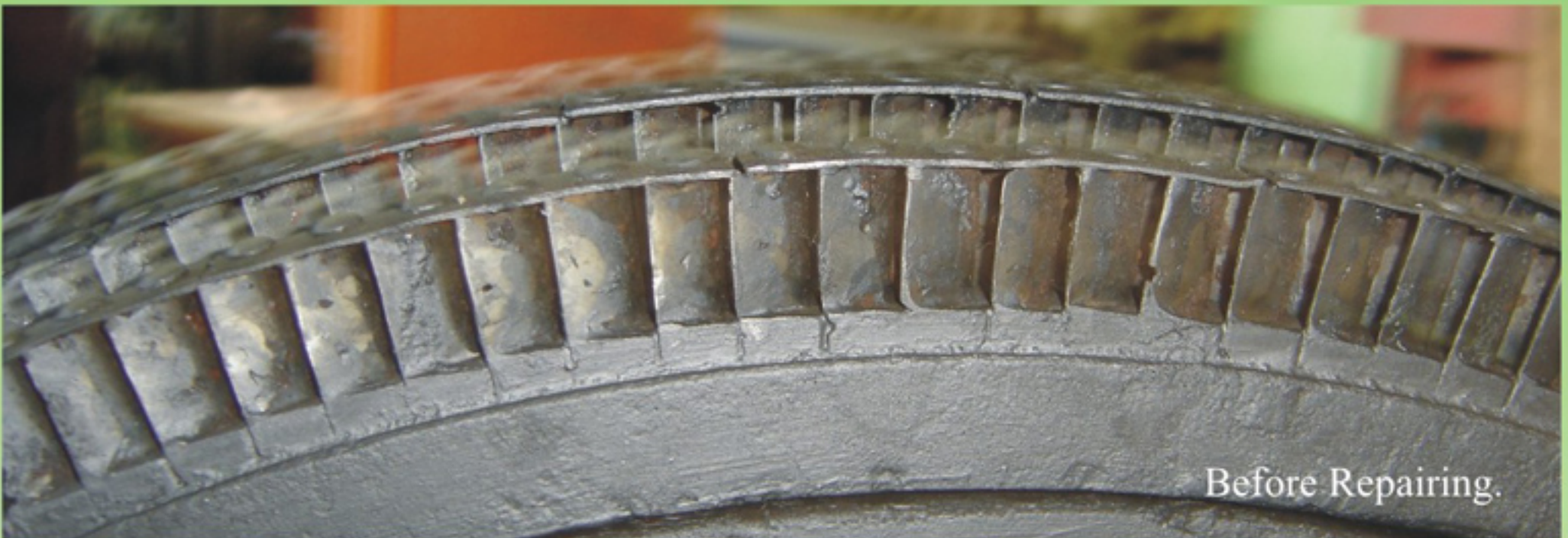
Worn out blades in American turbo dyne turbine rotor.
