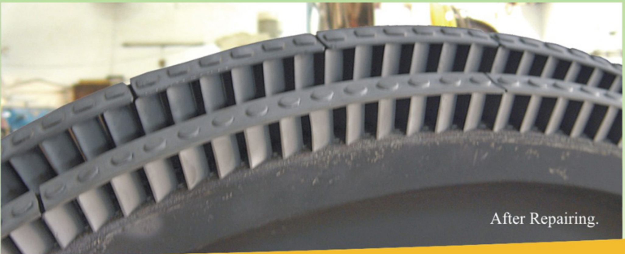
Worn out blades in American turbo dyne turbine rotor.
