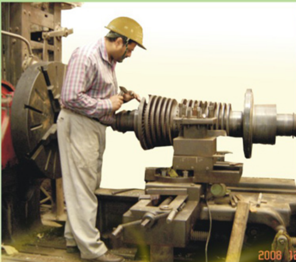
Power House 10 MW Turbine Rotor blade fitting in process
