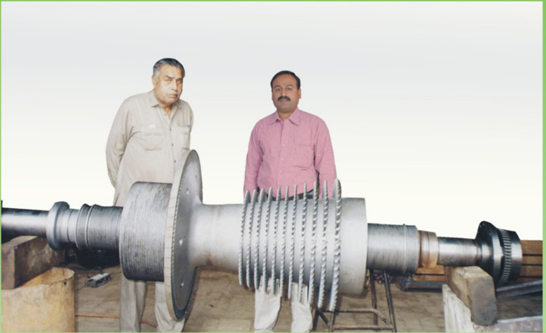
Power House 10 MW Turbine Rotor blade fitting in process
