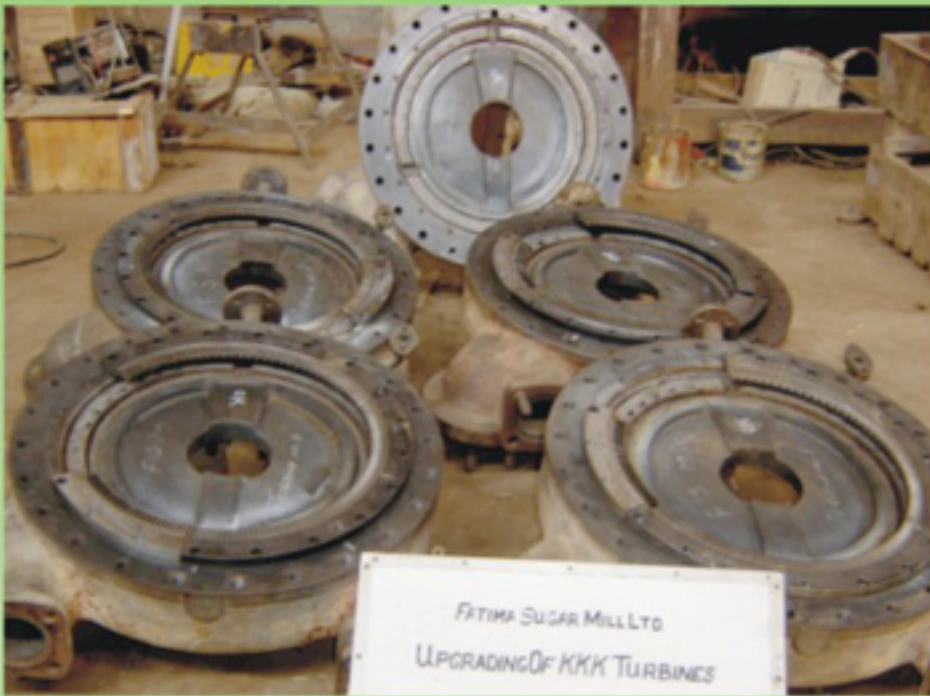
New first stage nozzle fitting into turbine body
