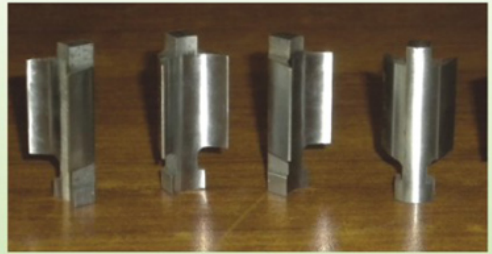
New blades that used in American turbo dyne turbine rotor.
